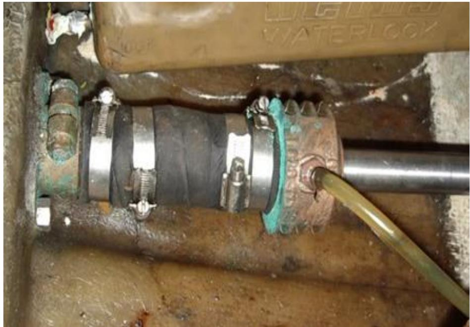
Subsequently, I have found that once at rest the stern glands are doing their job because they eventually seal out the ingress of seawater when the shafts are not revolving.
